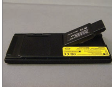
USB Receiver is stored in the back of the Express Card Presenter.
